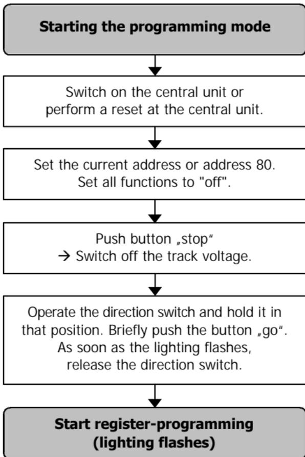
After having started the programming mode (and when the locomotive's lighting flashes) you can program the decoder's registers as follows:
